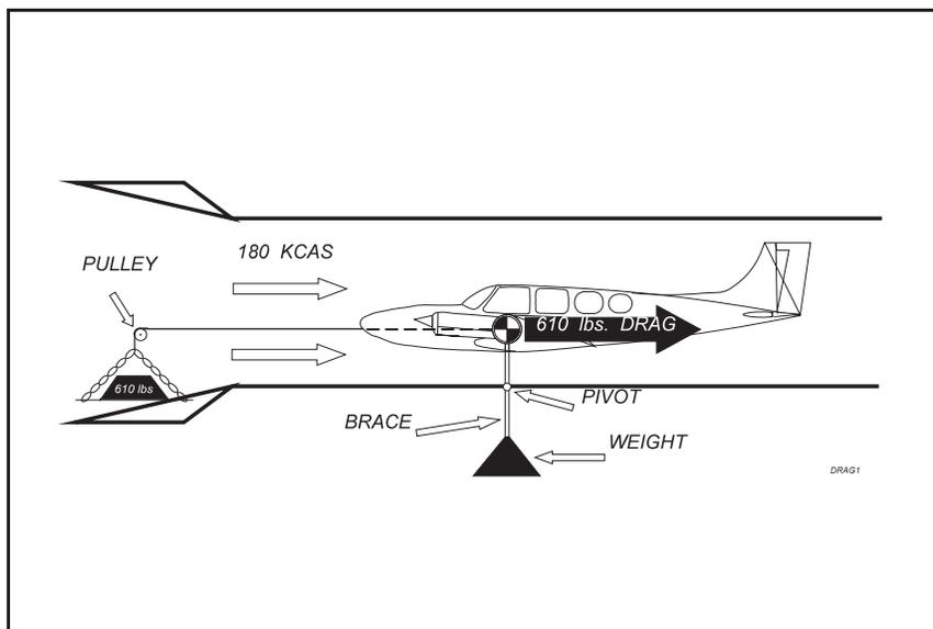
**Figure 2.** Measuring drag.
